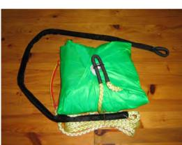
34 >> Fold the bridle a figure 8 and secure one end using the side rubber band. (replace it, if necessary). The deployment bag is now ready to be fitted into the harness, according to the
