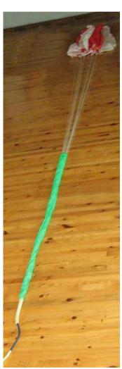
8>> Grasp all the suspension lines with one hand and check if all the knots are at the same height.
